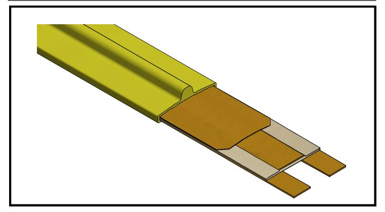
**S-33** type pressure sensitive ribbon switch is a safety device designed according to the European and Italian safety norms. It may have different length and it is housed inside the **Proswitch™** sensing edges.
