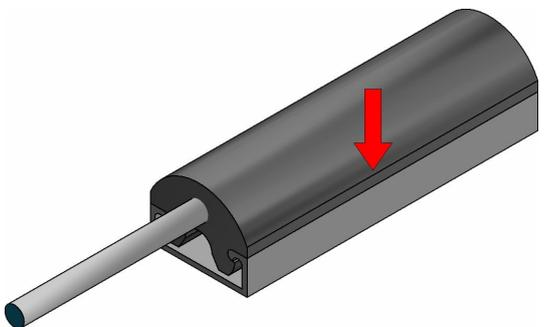
Insert the other side of the edge housing, pushing it down without putting too much pressure on it.
