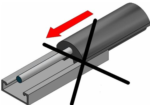
**NB:** never insert the edge housing by making it roll on the edge channel longitudinally. This may cause irreparable damages to the edge housing and to the sensor reliability.
