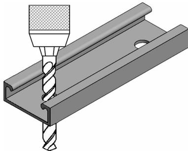
If the machine has not the profile section, the aluminium edge channel should be installed by drilling evenly holes along the edge channel, keeping a reasonable distance between 200 mm and 300 mm.
