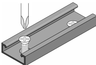
Once the flared holes are done and cleaned from eventual drilling traces, you can insert the appropriate screws.
