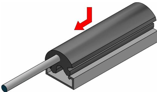
Apply the edge housing on the edge channel, starting inserting it carefully from one side.
