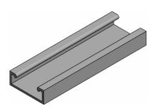
Aluminium edge channel is the support that allows the installation of the edge housing on the machine. It is designed to ensure a proper assembly of the sensing edge. Otherwise, it is possible to fit the aluminium edge channel directly to the machine profile section, in order to reduce the time requested for the installation and to respect the machine design.
