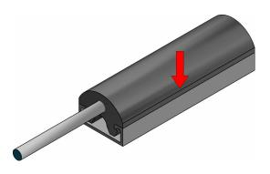
Insert the other side of the edge housing, pushing it down without putting too much pressure on it.
