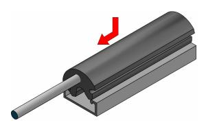
Apply the edge housing on the edge channel, starting inserting it carefully from one side.
