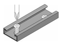
Once the flared holes are done and cleaned from eventual drilling traces, you can insert the appropriate screws.
